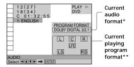
\* "PCM," "DTS," "DOLBY DIGITAL" or "MPEG" is displayed. In case of "DOLBY DIGITAL," the channels in the playing track are displayed by numbers as follows:
